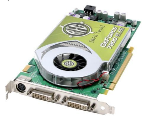
The model designation contains the characters "OC", suggesting that the card is a factory overclocked product. Its core frequency is 425MHz – the same as the flagship GeForce 7800 GTX and 25MHz advanced from the stock 7800 GT card. The memory data rate is 1050MHz – also a little faster than the stock 1000MHz. These clock speeds should help push the card's
